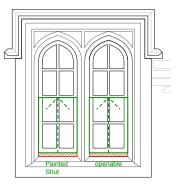
Ref: 1W01 Location: Police Station, First floor Type Existing: Timber framed double hung single glazed sash windows Proposed Works: Rotten cill to be replaced in new hardwood, Rake out dead and defective putties and replace in linseed oil putty, cut out swollen joints and repair using window care repair if required. Sash cords, weights, staff beads & parting beads to be refurbished where required. Window and subframe to be prepared, with painted finish Repair Code: Code: 3 Glazing: Not Required
