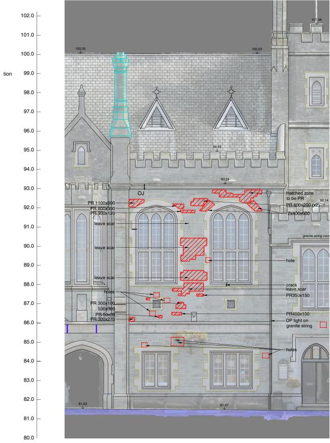
**Tabric Repair to South West Elevation**Scale 1:100
