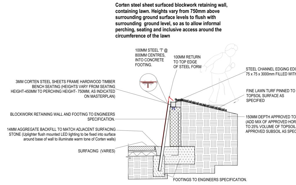
Hardwood timber bench with backrest recessed into Corten furnished lawn retaining wall (450mm - seating height) high (see detail below)
