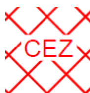
Figure 2.08 – Example used on the TPP to indicate the location of CEZ, as shown in this figure.
