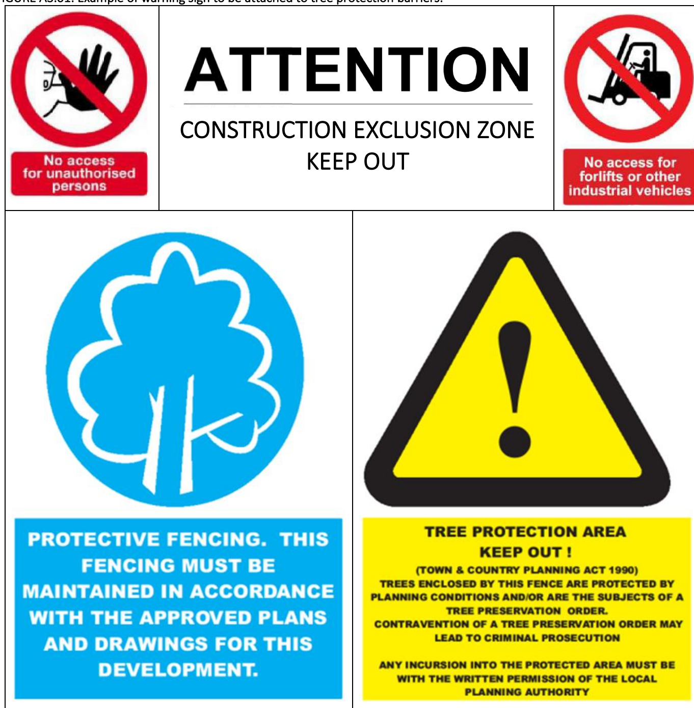
FIGURE A3.01: Example of warning sign to be attached to tree protection barriers.
