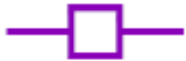
Figure 2.06 – Example used on the TPP to indicate the location of special measures required, as shown in this figure.
