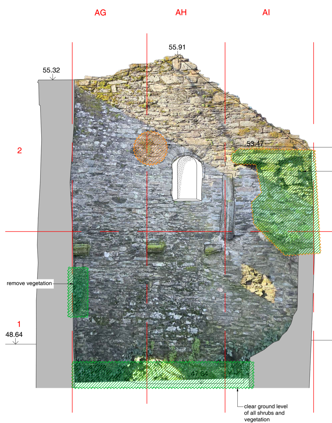
02 North West Internal Elevation - Proposed Fabric Repairs Scale 1:50
